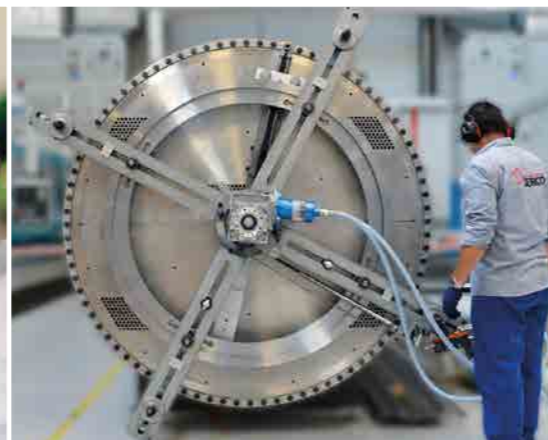
> Portable machine tools for maintenance and repair of flanges and valves.
