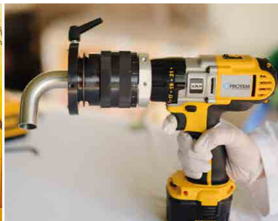
> PROTEM tube squaring machines enable a perfect surface with no rough edges.
