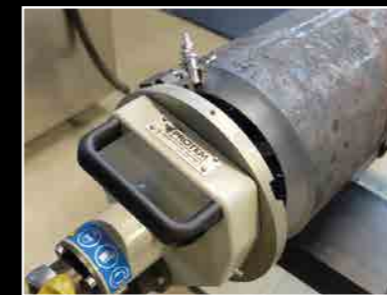
> PROTEM machines from the US Series, which allow preparation for perfect quality welding
