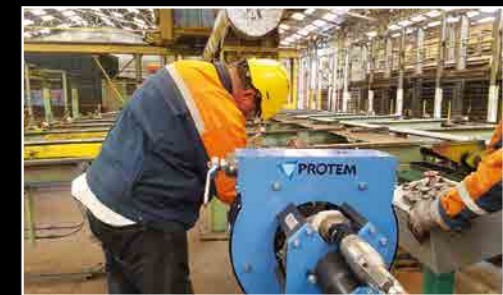
> PROTEM BMFM mobile beveling bench, for machining high thickness tubes
