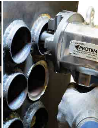
> Removing welding seams for extubation operations using the PROTEM US30CH tube beveling machine
