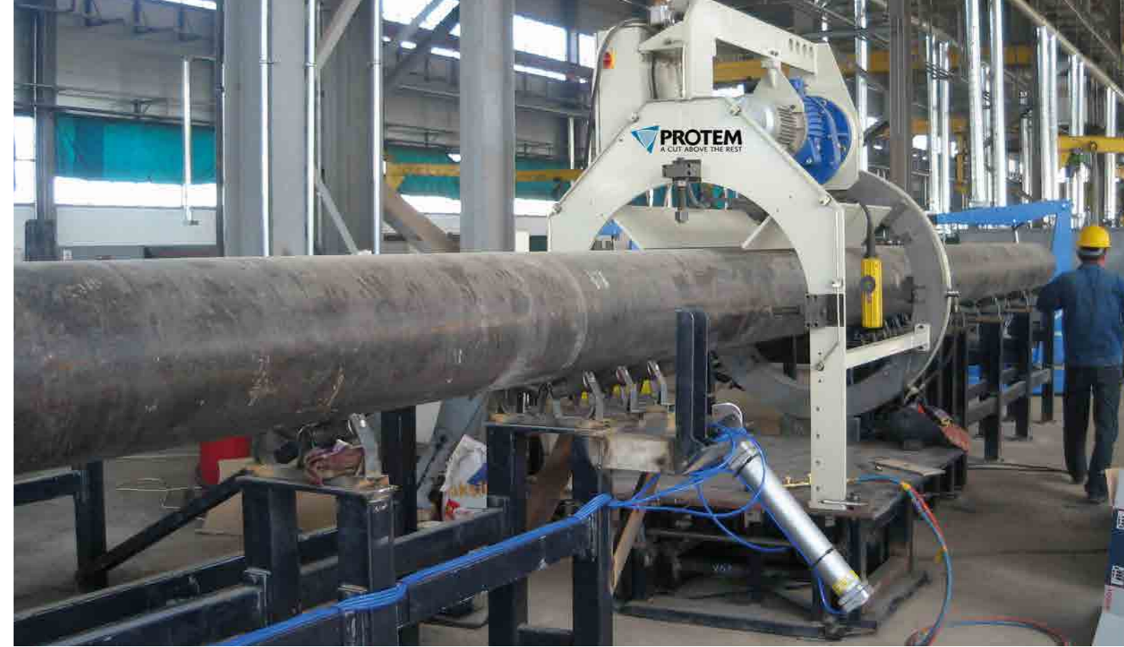
> Prefabrication of tubes on-site or in the workshop, with a PROTEM TNO cutting and beveling machine
